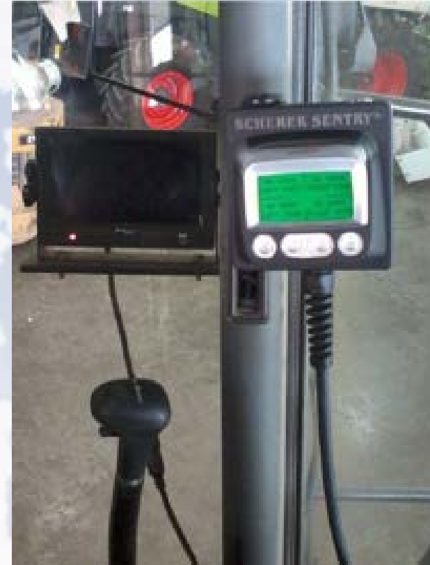
Cabin monitoring of bearing temp. and air pressure
